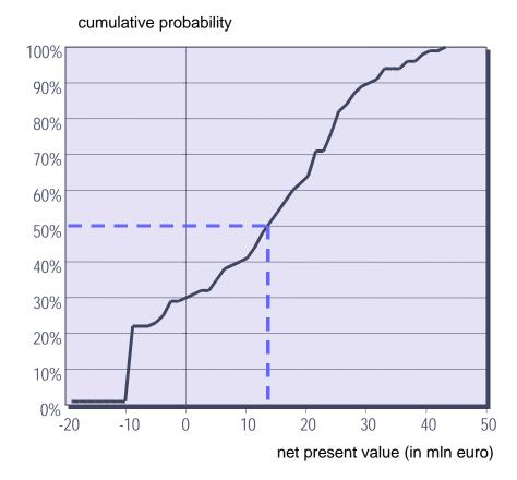
Figure 3.3 Example of the probability distribution for the net present value of a renewable energy project based on a Monte Carlo approach. The expected value (P=50%) is 14 mln Euro. The Value-at-Risk(VaR) is 24 mln Euro in this case (VaR = NPV(50%) – NPV(10%) = 14 – (-10) = 24 mln. The analysis also shows that this investor has 30% probability of not meeting his internal financial return targets (NPV < 0).</li>
