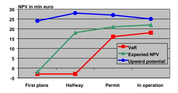
*Figure 3.5* Value-at-Risk (VaR), expected NPV and upward potential estimated using a Monte Carlo approach for the development of a wind farm with 20 turbines in the Netherlands
